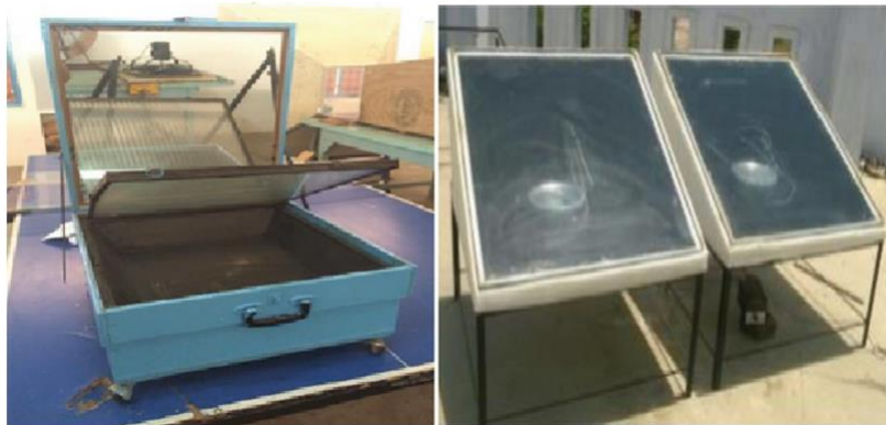
Abb. 4 Konventioneller box type solar cooker.
